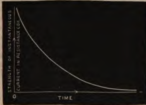
Curve representing the Discharge of a Condenser through a Large Resistance. Discharge Unidirectional and Continuous.
